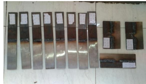
Fig 1. Dissimilar metals welded before breaking
